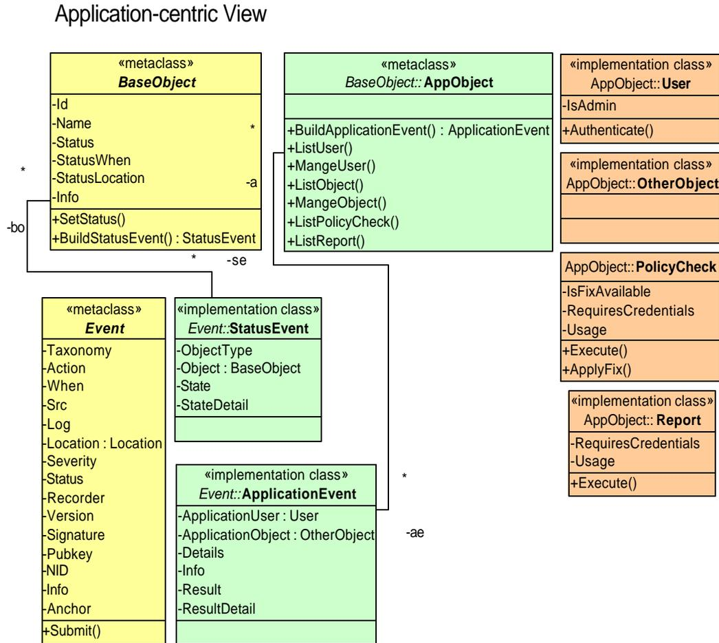
Figure 12 – Application-Centric View
